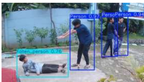
Figure 25. Detection of a Fallen Human Object (fallen_person) with a Confidence Score of 0.76.
